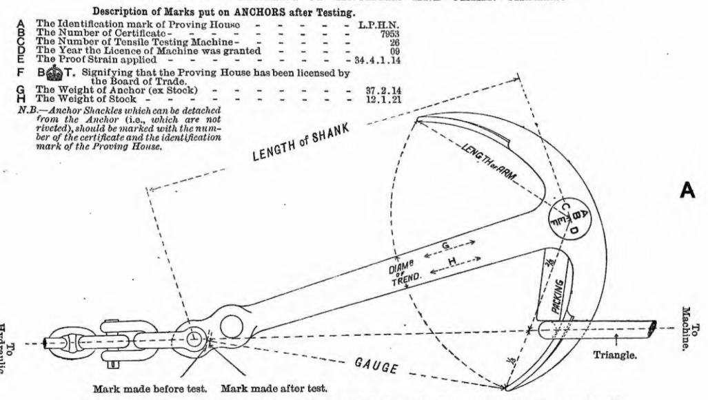
The difference between the positions of the marks made before and after testing to be not more than 3".
