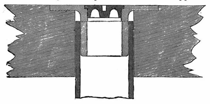
at the decks. The accompanying sketch shows approved arrangements for the connection of such pipes.
